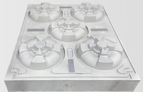
A cast- to-size mold to form a returnable dunnage tray
