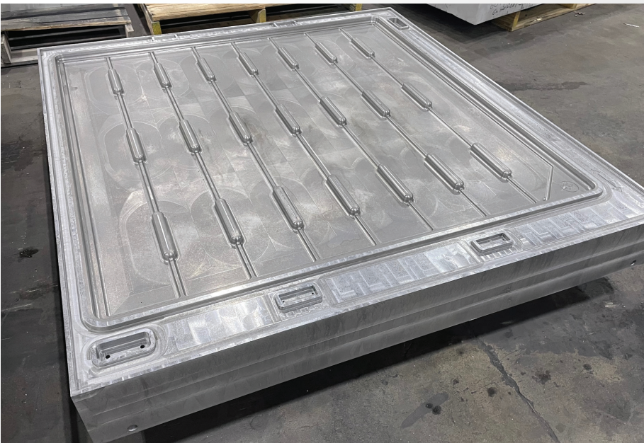
A “cast oversized and machined” mold for a floating dock.
