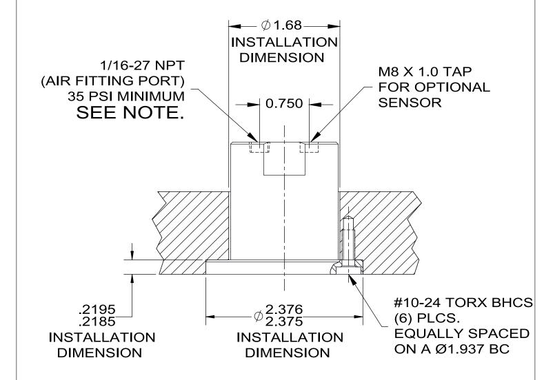
**NOTE**: WHEN INSTALLING 1/16-27 AIR FITTING DO NOT EXCEED TWO FULL REVOLUTIONS. EXCESSIVE FITTING ENGAGEMENT CAN INTERFERE WITH THE CYLINDER LOCKS ABILITY TO ACTUATE PROPERLY, CAUSING IT TO MALFUNCTION!
